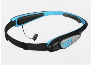
(a) The BrainLink Pro single-channel EEG headset.
